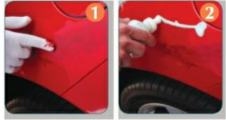
The scratch is cleaned and the patented SSR base paint colour is applied.
